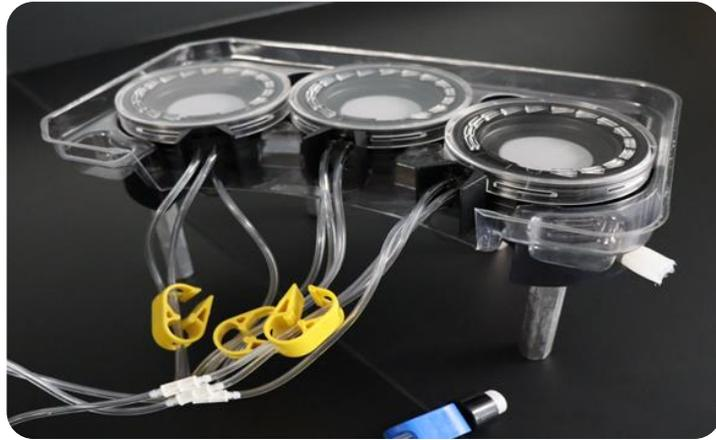
An FDA required sterility test performed by manufacturers before final product can be released for commercial sale
